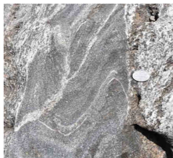
Fig. 15. Valanthode SHEP: Ptygmatic folds seen in the migmatited gneiss in the eastern section of weir axis.
