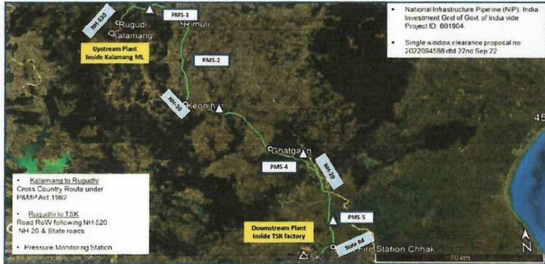
Fig-2: Layout of Slurry Pipeline from Kalamang to Tata Steel Kalinganagar
