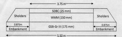
SDBC: Semi-Dense Bituminous Concrete WMM: Wet Mix Macadam GSB: Granular Sub-Base
