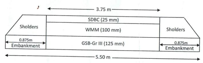
SDBC: Semi-Dense Bituminous Concrete
