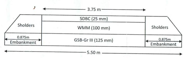
SDBC: Semi-Dense Bituminous Concrete
