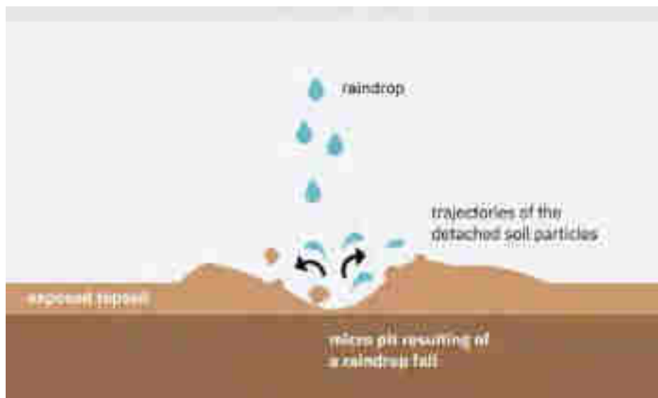
Fig No. 2.1: Figure showing splash erosion
