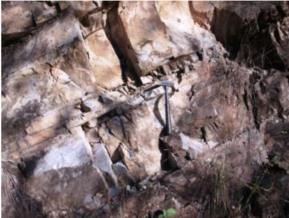
Photo-11: Very hard, medium grained limestone at left abutment, above the dam axis.
