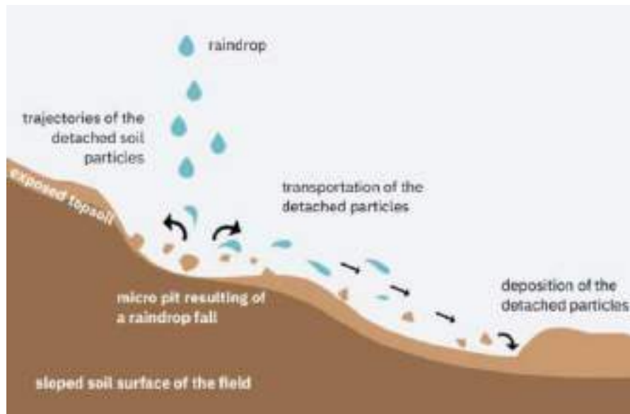
Fig No. 2.2: Figure showing stages of soil erosion processes
