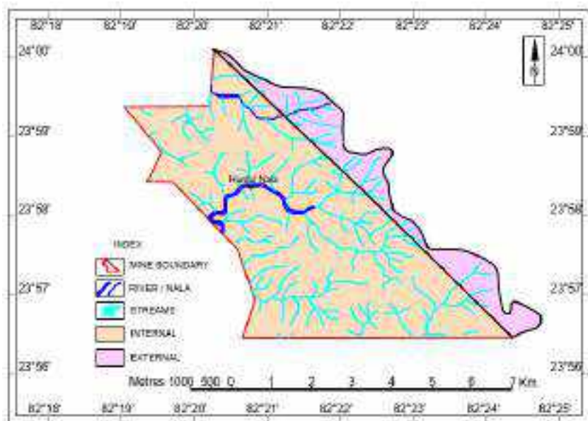
Figure 27: External and Internal Mine watershed
