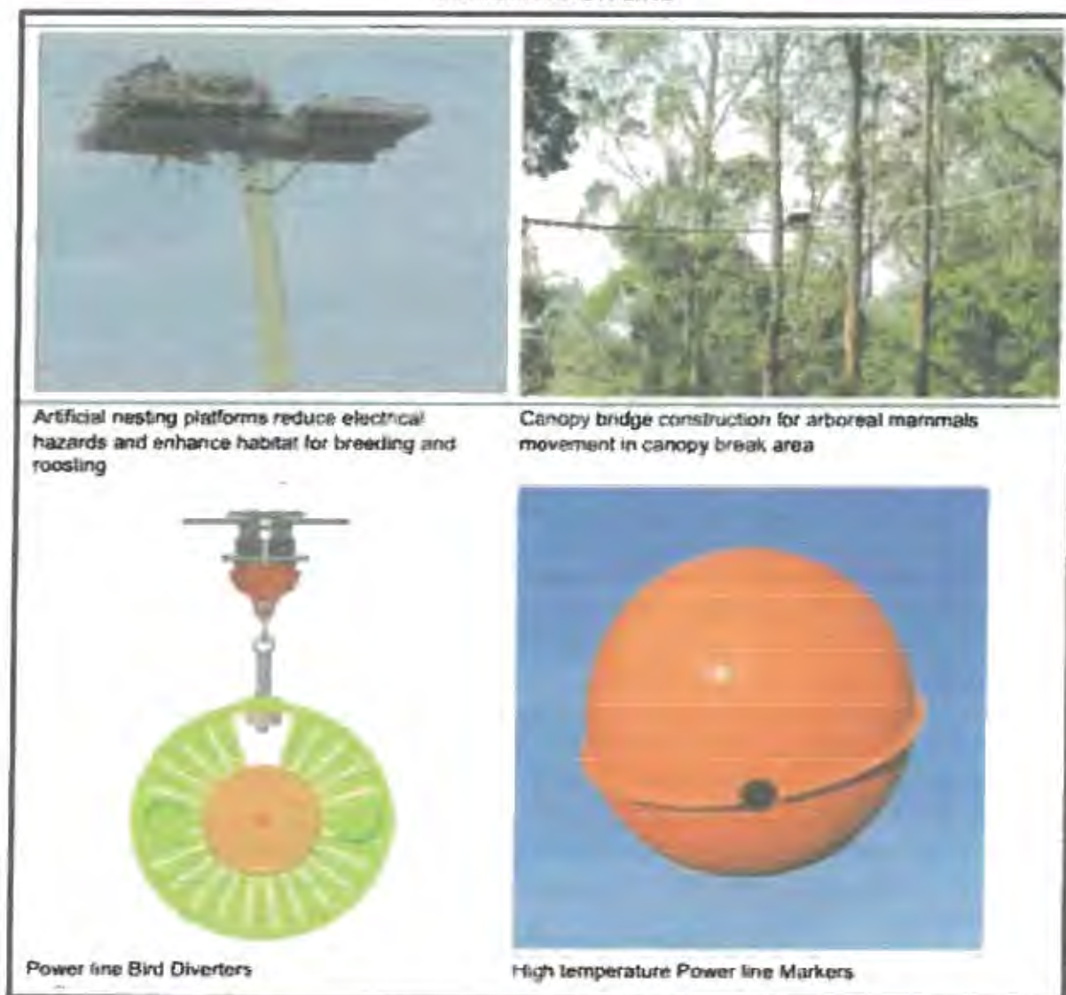
FIGURE 4.A.1: WILDLIFE PROTECTION DEVICES/STRUCTURES FOR PROPOSED TRANSMISSION LINE
