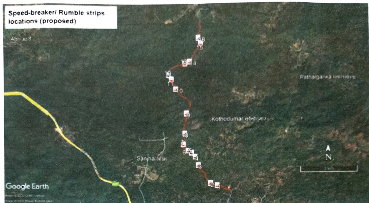
Figure 2: Sixteen (16) locations along the PMGSY road where installing effective speed-barriers in the form of speed-breaker and/or rumble strip pairs are proposed to reduce vehicular speed thus minimising animal-vehicular collision risks
