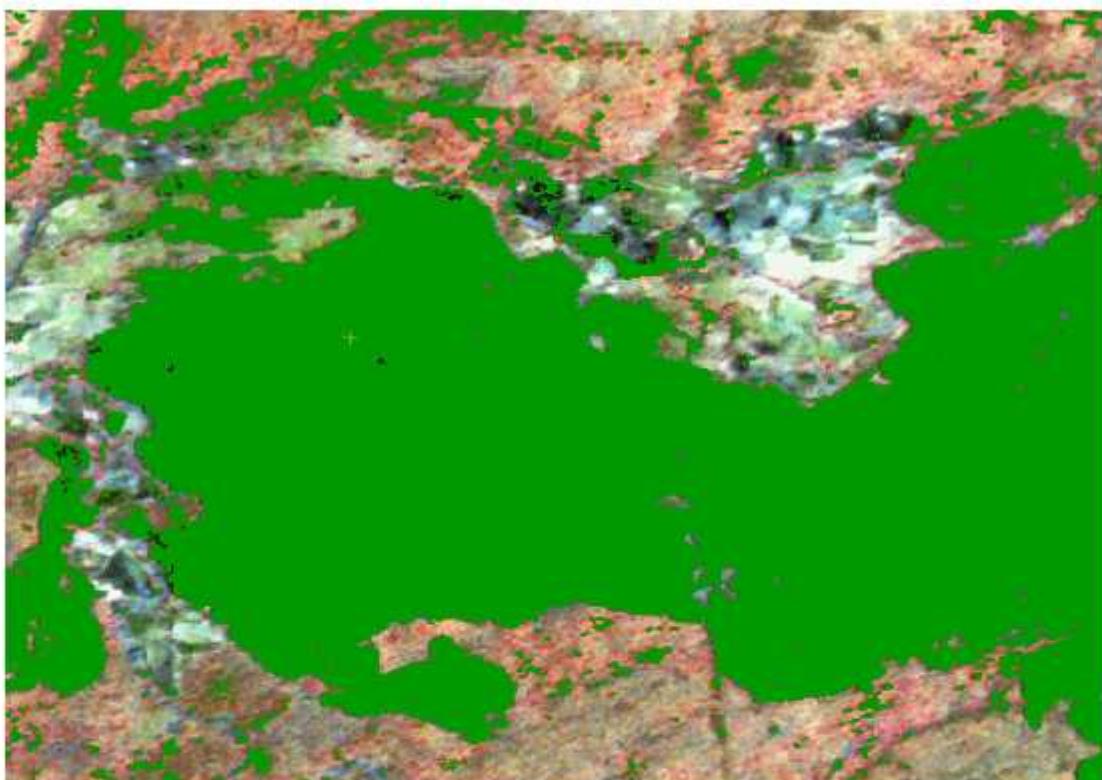
Figure 2.2: Extracted forest cover from IRS P6 LISS IV Satellite Image by the method of Spectral Reflectance Analysis
