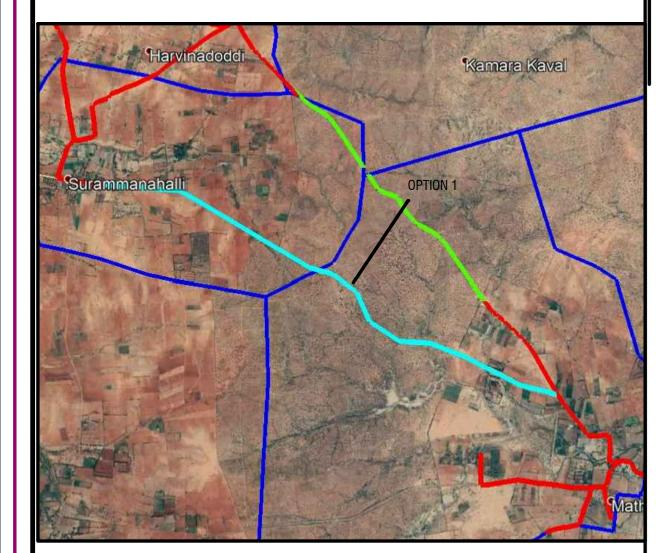
In this reach we have examined the alternate alignement to aviod the forest area, Firstly it was proposed to as per Option 1 alignement. After Knowing the alignment is passing through the forest area, the alignment is changed and reduced the forest area and final some reach is crossing through the forest area as shown
