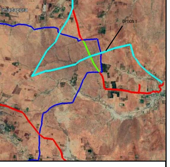
In this reach we have examined the alternate alignement to aviod the forest area, Firstly it was proposed to as per Option 1 alignement. After Knowing the alignment is passing through the forest area, the alignment is changed and reduced the forest area and final some reach is crossing through the forest area as shown in above
