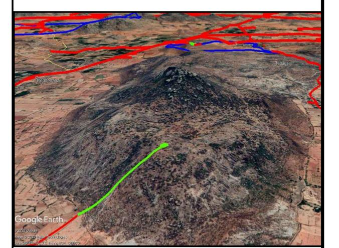
Proposed pipe line and Water Tank (GLSR) is very essential to locate at elevated location of hilllock, so as to provide the water through gravity and less pumping cost can be achived
