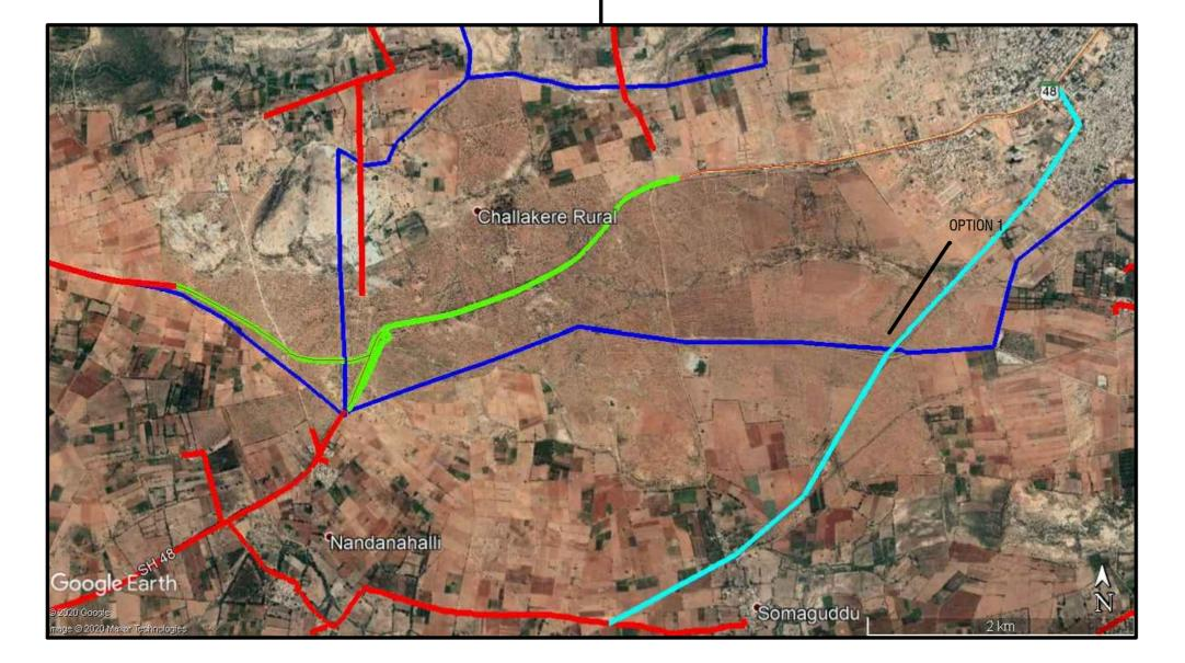
In this reach we have examined the alternate alignement to aviod the forest area, Firstly it was proposed to as per Option 1 alignement. After Knowing the alignment is passing through the forest area, the alignment is changed and reduced the forest area and final some reach is crossing through the forest area as shown in above
