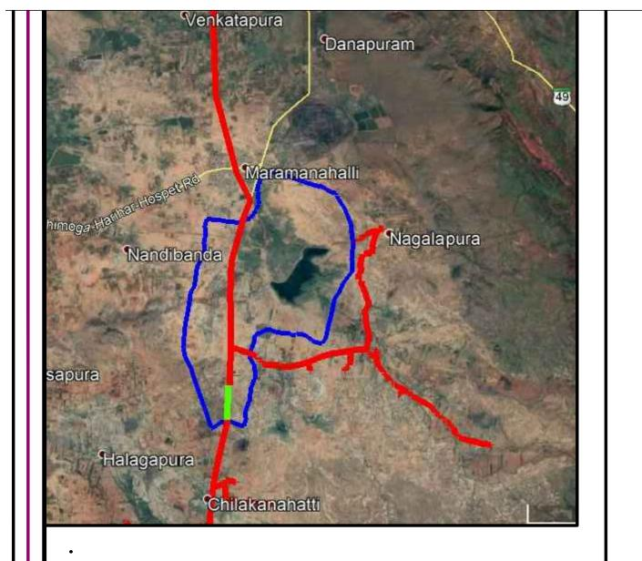
1. Pipe Line Alignment of Raw Water Rising Main is Passing through Forest Area for 965 m, There is No Possibility for exmain the other alternate as shown above
