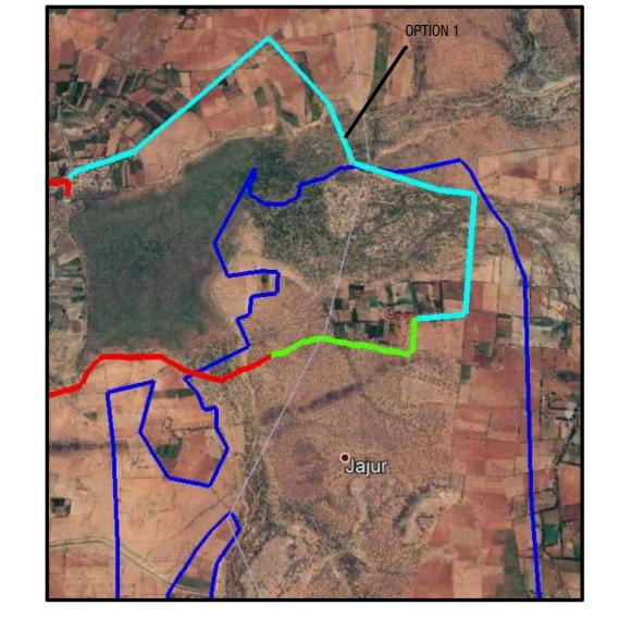
In this reach we have examined the alternate alignement to aviod the forest area, Firstly it was proposed to as per Option 1 alignement. After Knowing the alignment is passing through the forest area, the alignment is changed and reduced the forest area and final some reach is crossing through the forest area as shown in above
