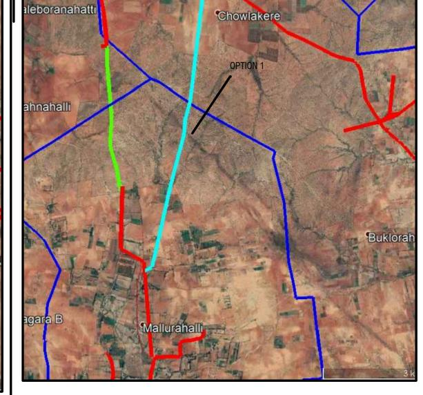
In this reach we have examined the alternate alignement to aviod the forest area, Firstly it was proposed to as per Option 1 alignement. After Knowing the alignment is passing through the forest area, the alignment is changed and reduced the forest area and final some reach is crossing through the forest area as shown in above
