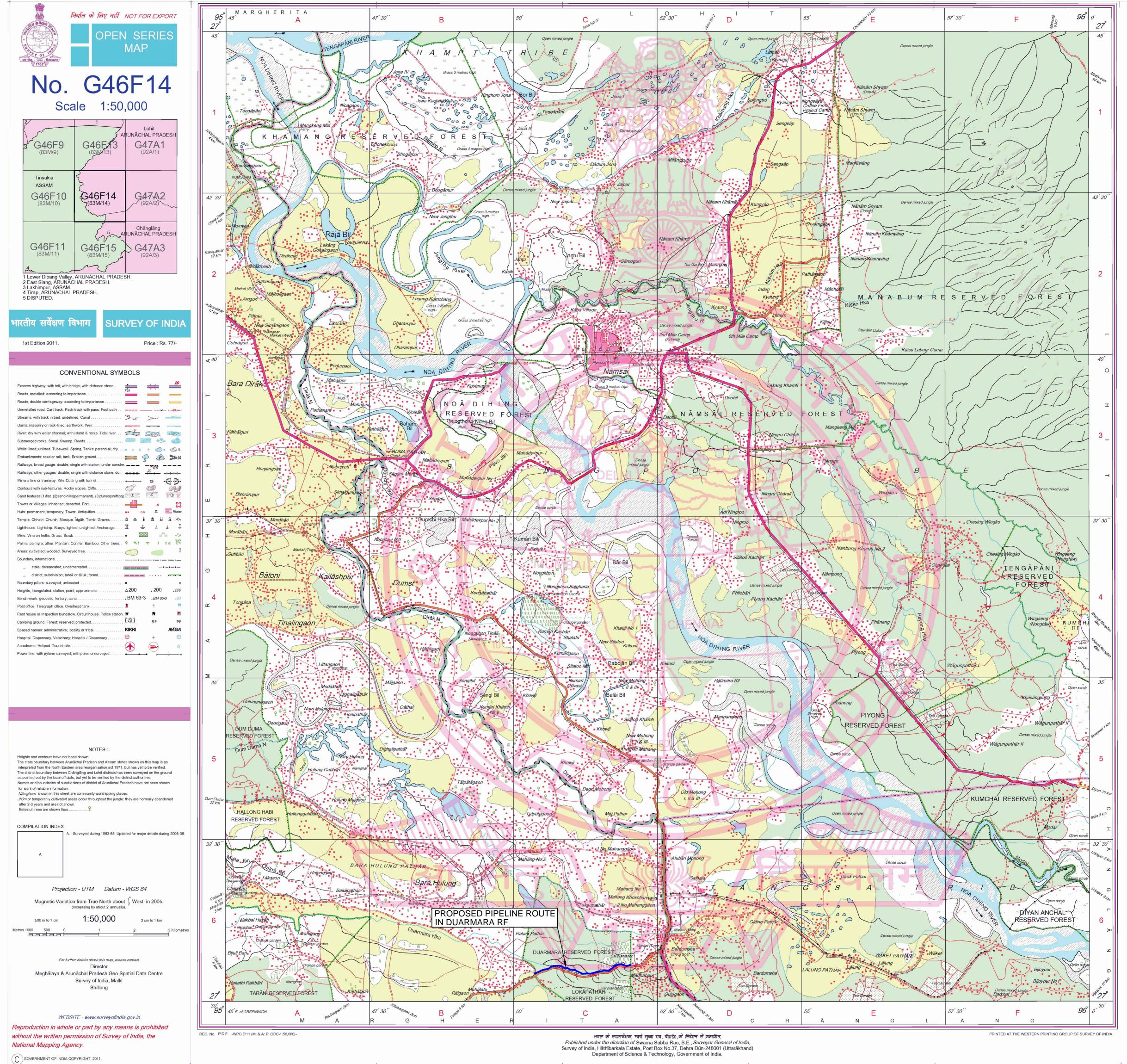
LENGTH OF PROPOSED PIPELINE IN DUARMARA R.F. 2.947 KM WIDTH OF PIPELINE CORRIDOR 15 MTS AREA UNDER DIVERSION OF FOREST 2947.07 X 15 = 44206 SQM AREA UNDER DIVERSION OF FOREST 2947.07 X 15 = 4.42 HA
