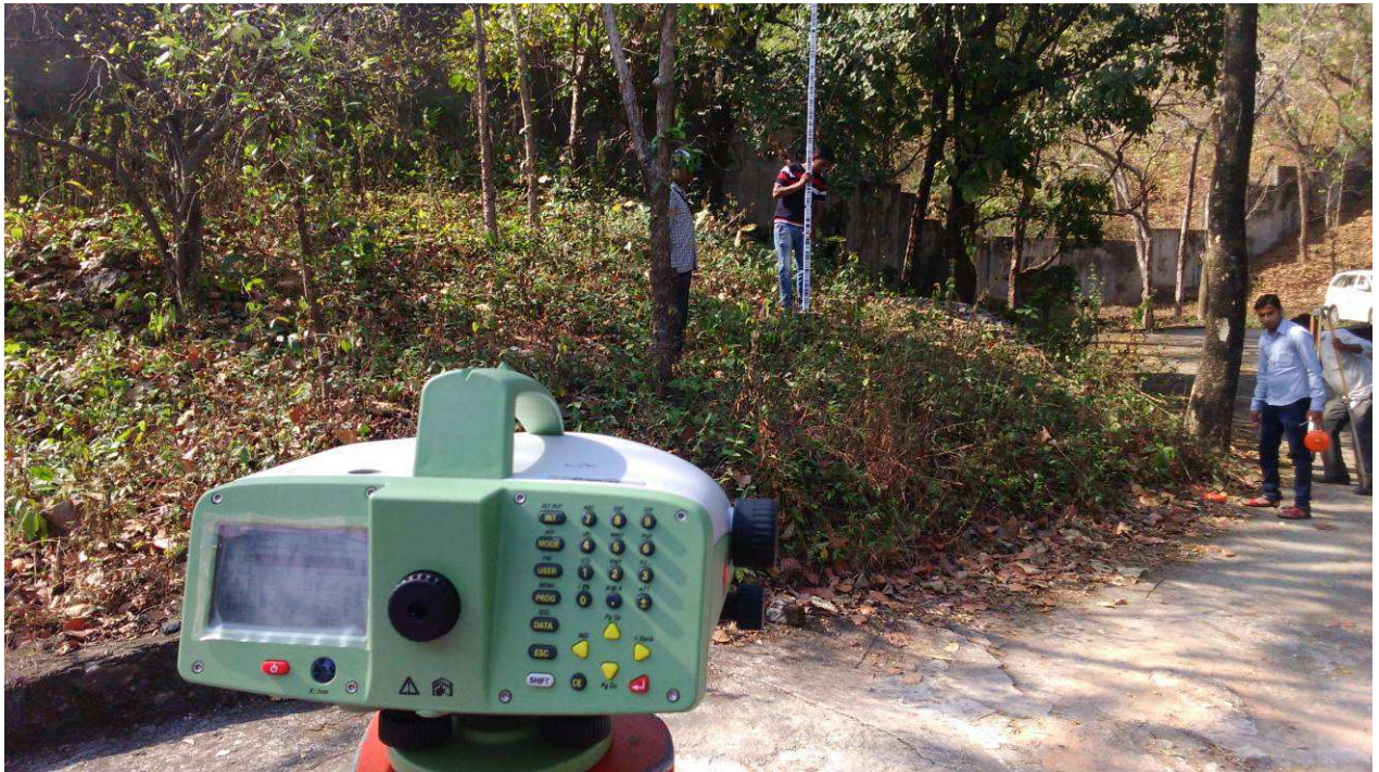
Fig. 13a: Monitoring of elevations at subsidence monitoring stations using precise digital level
