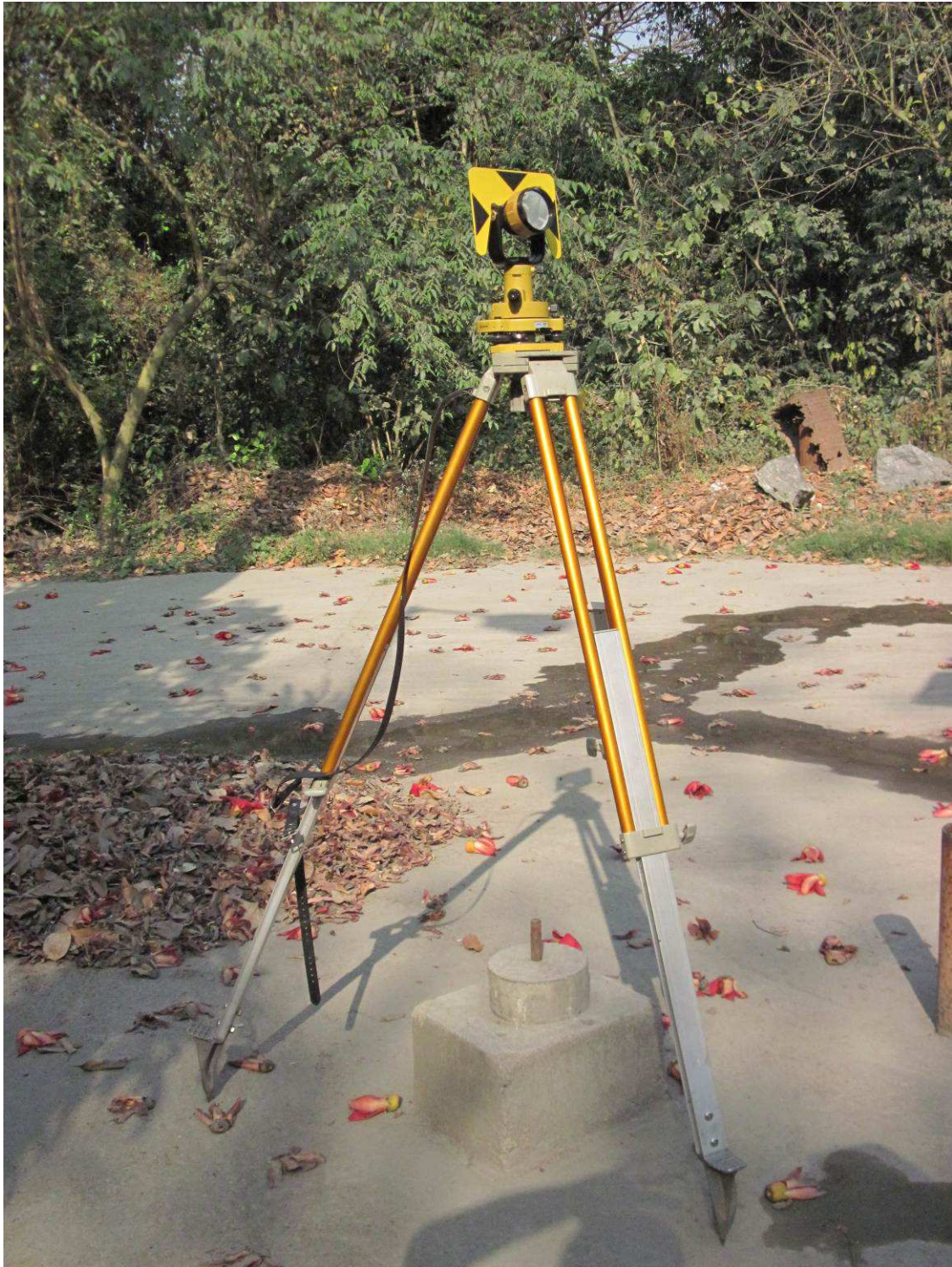
Fig. 11: Monitoring of coordinates (x, y) over the permanent subsidence monitoring station using Prism monitoring (EDM) at D6
