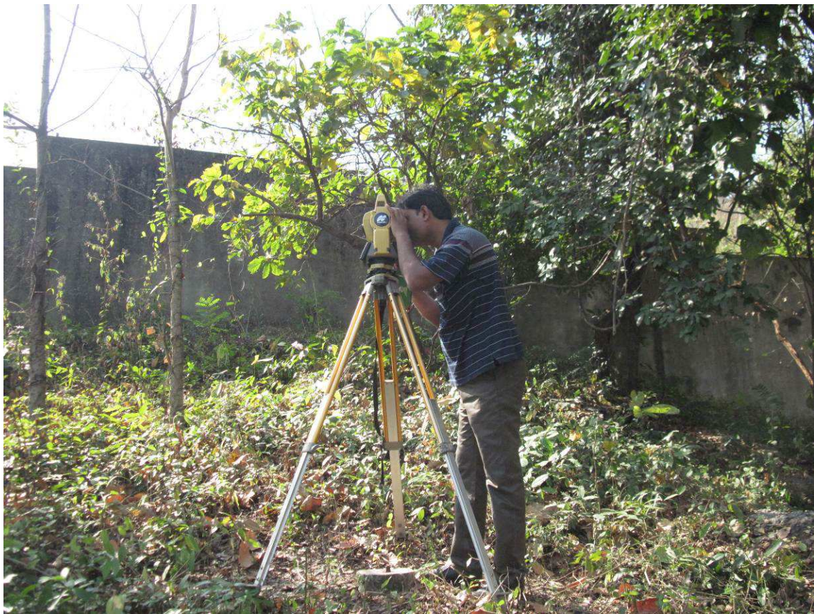
Fig. 12: Monitoring of coordinates (x,y) over the permanent subsidence monitoring station in the forest area using total station
