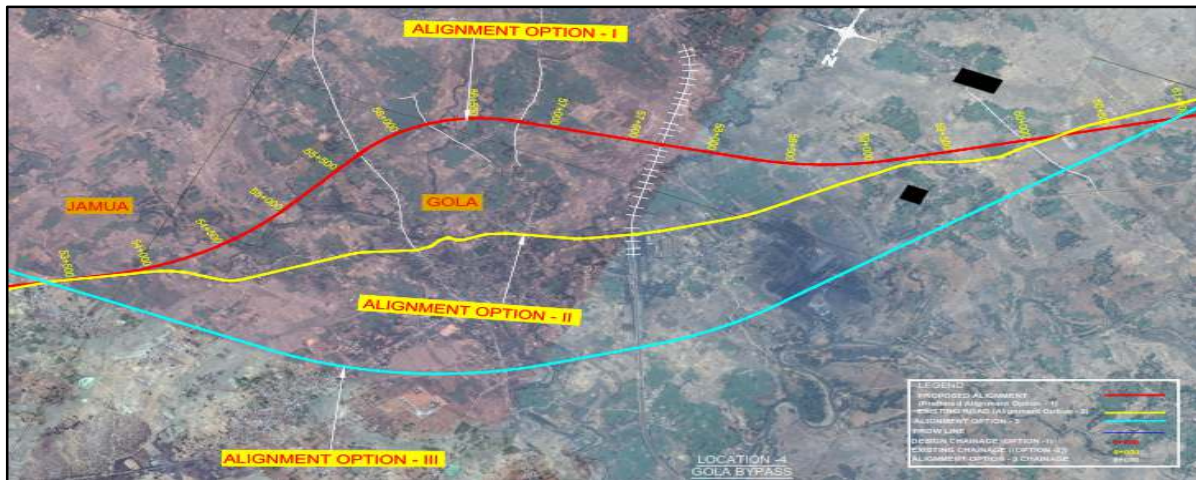
Fig- Alignment Option Map(L4) proposed at Gola
