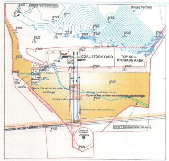
Data is available in two bore holes in area south of proposed quarry. Stripping ratios are 21.94 and 22.71. From trend of stripping ratio lines, it is evident that south of proposed quarry area is uneconomical. However, if in future, part of this area becomes economical, receiving hoppers, coal stock yard and top soil storage area will be re-located for whatever coal can be extracted.
