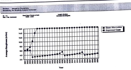
Figure 7: Roughness of Mangan to Chungthang (2024-2050)
