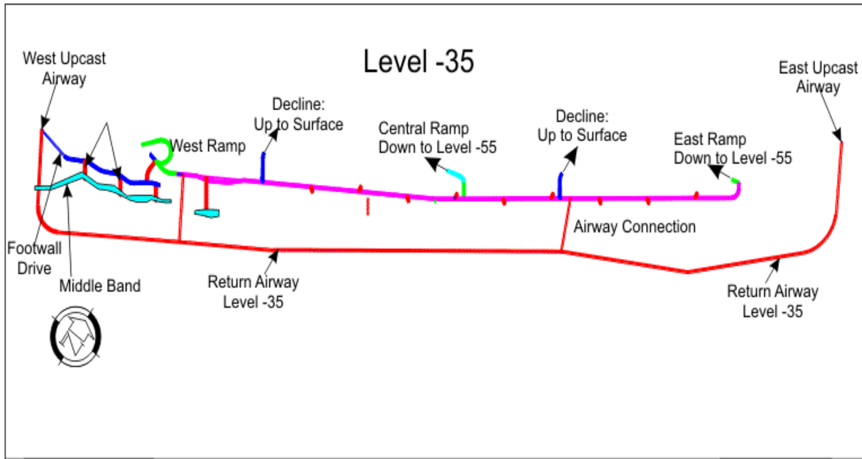
Fig. 4.15: Schematic Mining Layout of Drive at Level -35 mRL
