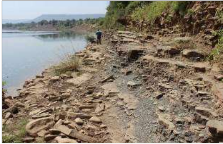
Photo 7: Alternate Shale & Sandstone Sequence along River Kuno - Right Bank
