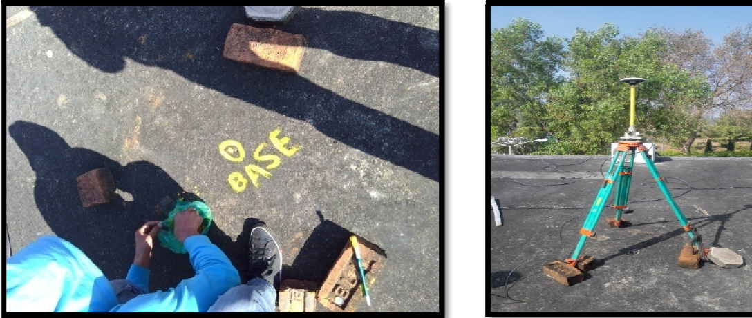
Fig-3: Images showing Primary Control Point (PCP)
