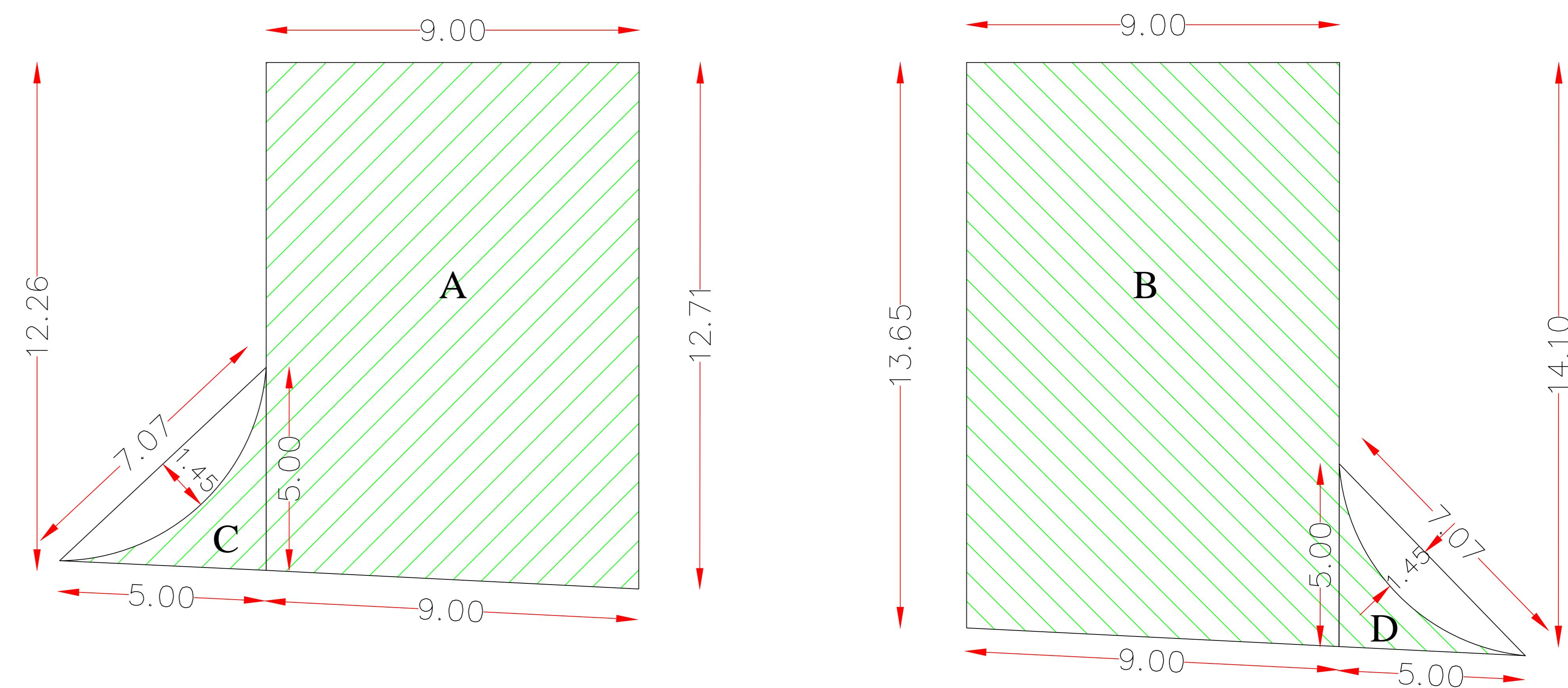
$$\begin{aligned}\text{AREA 'A'} &= 9.00 \times \frac{1}{2} (12.26 + 12.71) \\ &= 112.36 \text{ SQ. MT.}\end{aligned}$$
