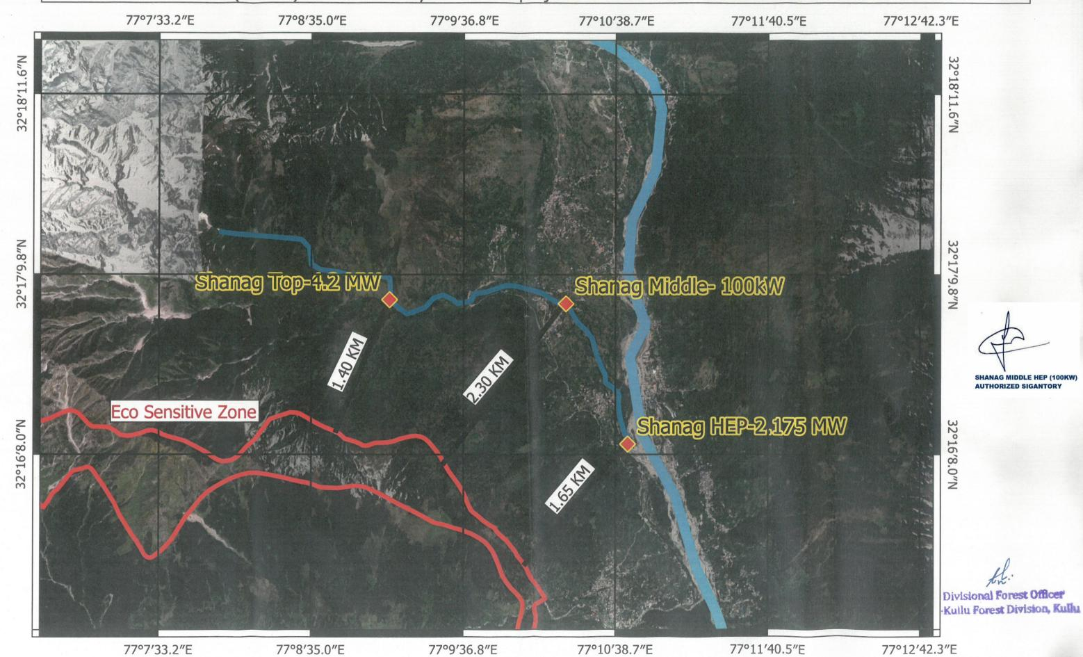
Georeferenced Map showing the distance from the Protected Areas and Eco sensitive Zones (ESZ) to Shanag Middle HEP(100kW) and all other hydro electric projects allotted in the Halindi Nallah Stream.
