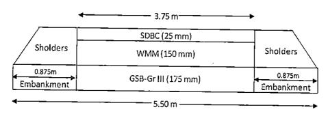
SDBC: Semi-Dense Bituminous Concrete
