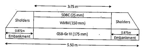
SDBC: Semi-Dense Bituminous Concrete
