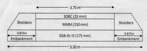
SDBC: Semi-Dense Bituminous Concrete
