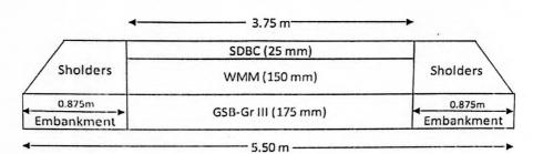
SDBC: Semi-Dense Bituminous Concrete
