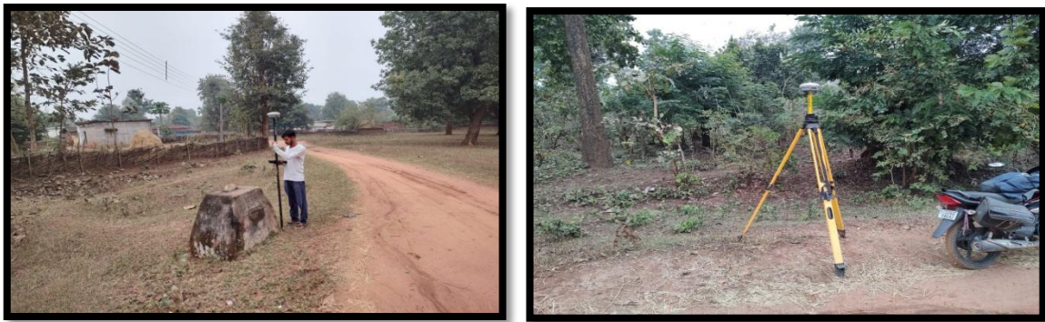
Fig. 4.1 A DGPS Base and Rover station Equipment
