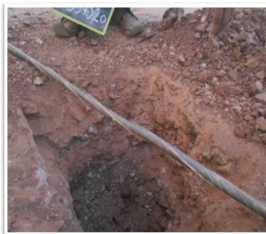
Photo : Existing Crust Thickness Survey
