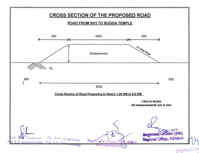
NAME OF THE PROJECT : ROAD FROM SH1 TO BUGGA TEMPLE TYPICAL PLAN SHOWING THE EXISTING AND PROPOSED ROAD ( Not to Scale) Forest Reach 1.26 KM to 5.6 KM. Existing Earthen Road width 4.00 mtrs (Average) Proposed Top width of the road Bottom width of the proposed road Bugga Temple 5.00 Mtrs 6.00 Mtrs 4.00 Mtrs 1/260 0/0 5/600 From Reach 1.26 KM to 5.6 KM = 4338.65 X 6/10000 = 2.6032 hectares 2.6032 hectares
