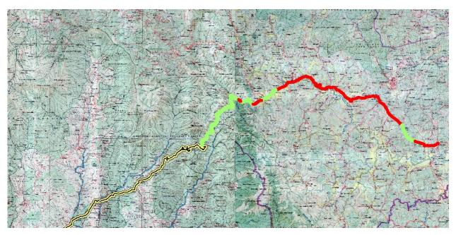
Project Cost: Proposed route from Ujire- Gonibeedu total length of 50 km in forest 1.013 Ha and m in nonforest area 0.76 Ha. Cost of laying of optical fiber cable is 500 rupees per meter and total project cost is about – 4 Crores
