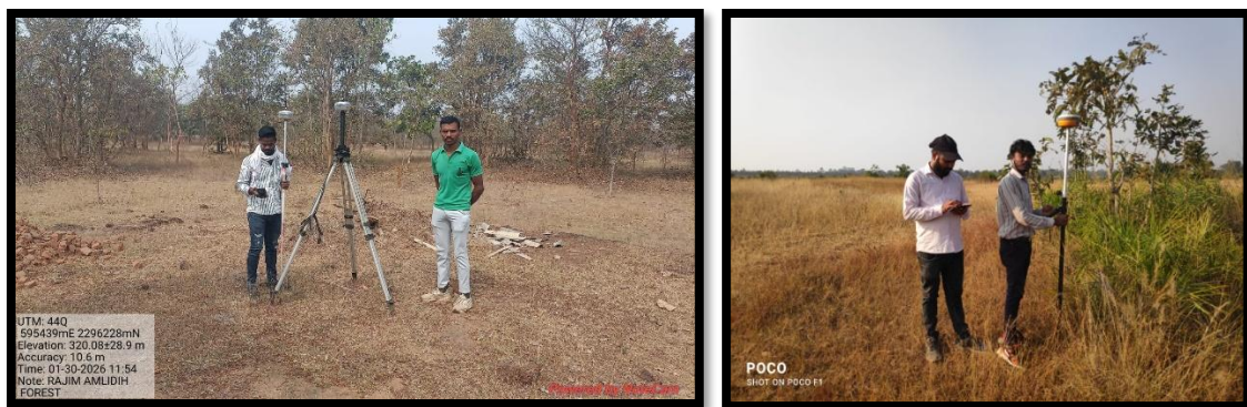
Fig. 4.1 A DGPS Base and Rover station Equipment
