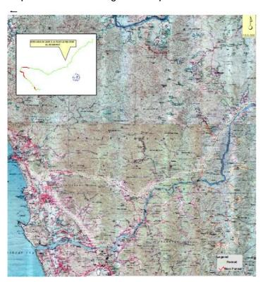
Project Cost: Proposed route from Ujire- Gonibeedu total length of 60.5 km in forest 1.539 Ha and m in nonforest area 0.2748 Ha. Cost of laying of optical fiber cable is 500 rupees per meter and total project cost is about – 3 Crores
