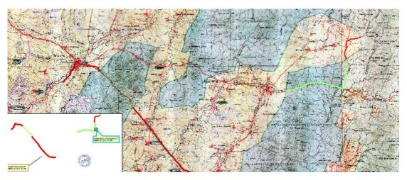
Project Cost: Proposed route from Kurahatti-Hanur total length of 34.5 km in forest 0.5487 Ha and m in nonforest area 0.48732 Ha. Cost of laying of optical fiber cable is 500 rupees per meter and total project cost is about – 1.5 Crores
