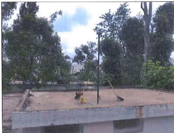
Fig-3: Image showing the establishment of the Primary Control Point
