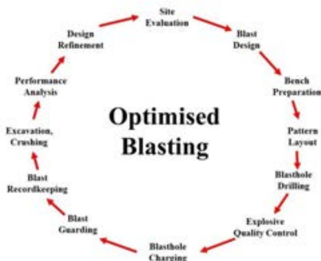
Figure 4.15: Optimized Blasting Cycle
