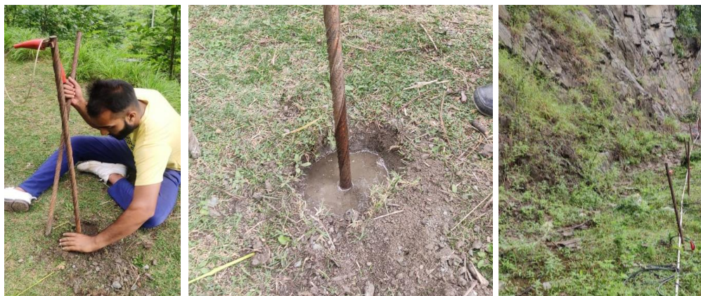
Photo 5.1 Electrode placement with clay, salt water mixture for better connectivity
