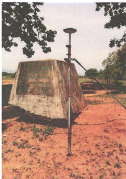
BASE STATION ON FOREST PILLAR AT KHAMARIA KHURD VILLAGE
