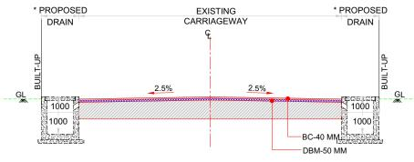
TYPICAL CROSS SECTION - 16B (FOR LEFT OUT BUILT-UP OVERLAY SECTION)
