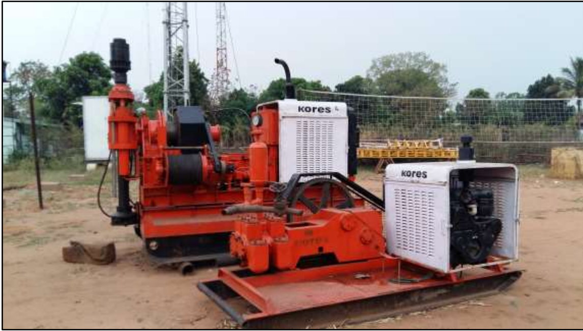
KORES KME 1000 DRILL RIG WITH L100C PRESSURE PUMP
