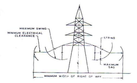
4.3 As per current practice, the width of RoW / corridor requirement for the transmission lines of different voltage levels are as follows.
