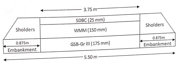
SDBC: Semi-Dense Bituminous Concrete
