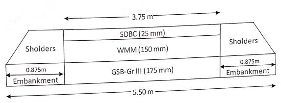
SDBC: Semi-Dense Bituminous Concrete
