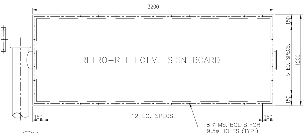
DETAIL SHOWING SIGN BOARD
