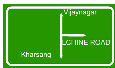
IS - 1 ADVANCE DIRECTION SIGN
