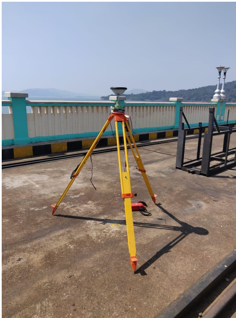
Figure 3 5: Reference bench mark considered is Supa Dam top level.
