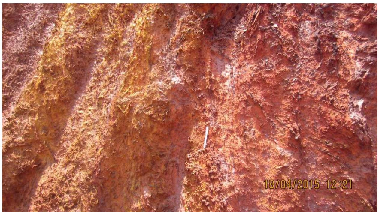
**Field Photo 2: Bench showing limonitic clay with limonitic ore near NW boundary of the lease area**
