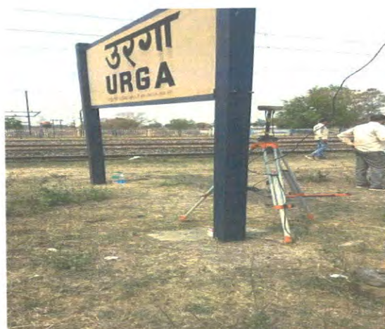
Fig-4: Photograph showing Urga Station Temporary Bench Mark (TBM)
