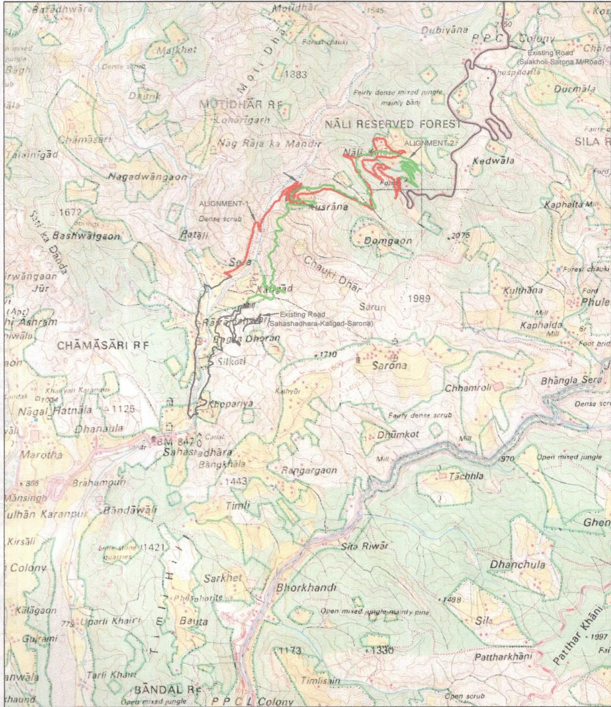
Alignment-1 shown in Red on Contour Map is Recommended for approval.
