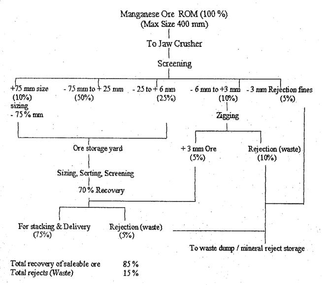
Note: All operations other than initial use of mechanical crusher are manual.
