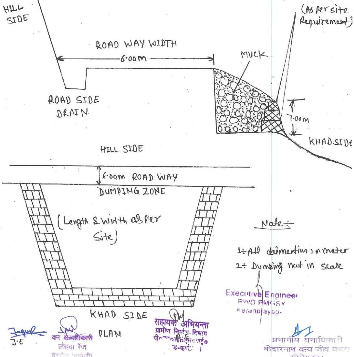
Name of Work : Muck Disposal Plan & Cross-Section
