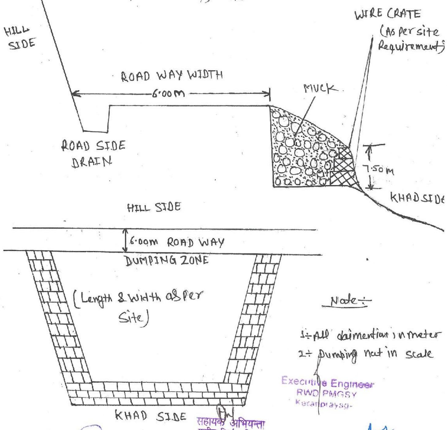
Name of Work : Muck Disposal Plan & Cross-Section
