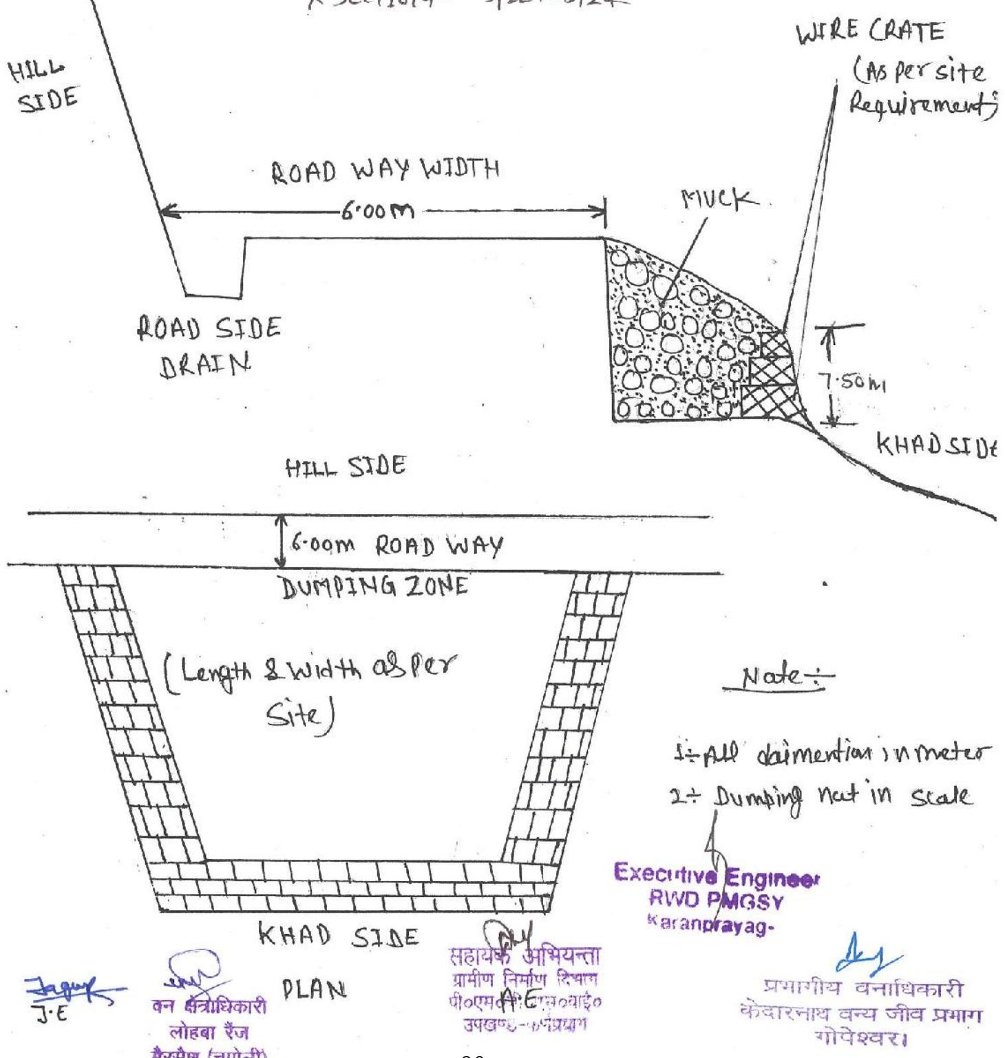
Name of Work : Muck Disposal Plan & Cross-Section
