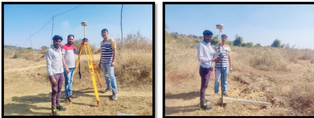
Fig. 4.1 A DGPS Base and Rover station Equipment
