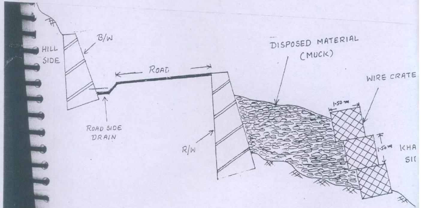
TYPICAL X-SECTION OF MUCK DISPOSAL PLAN
